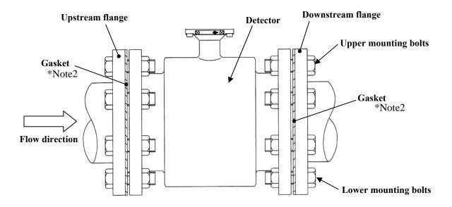
Figure 4.5 GF63\* flowmeter detector piping connections
